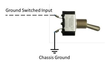
It is very important that you are only connecting ground to the inMOTION NGX inputs. Do not connect positive voltage to the inputs. This will damage the inMOTION NHX module and void the warranty.
